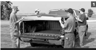
With Tail Gate Open and Using 4 Individuals, Place Tonneau Cover onto Truck Bed Rails.
