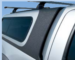
Spray-on protective coating increases strength in high stress areas
