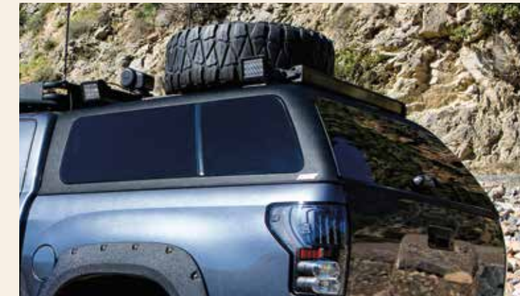
Spray-on protective coating increases strength in high stress areas.
